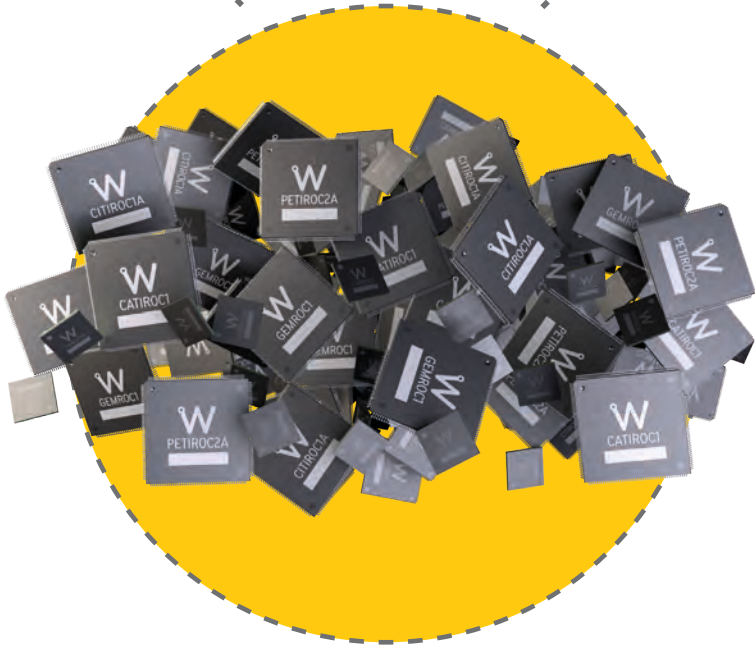
TEMPOROC Temporoc is a 64-channel front-end ASIC designed to readout silicon photomultipliers (SiPM) in particle time-offlight (TOF) measurement applications.
