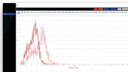
Energy spectrum measured at the two ends of one ^3\text{He} tube - x-axis is not-calibrated energy.
