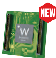
RADIOROC Radioroc is a 64-channel front-end ASIC designed to readout silicon photo-multipliers (SiPM).
