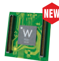
PSIROC Psiroc is a 64-channel front-end ASIC designed to readout PIN diodes, silicon strips and GEMs, handling detector capacitances ranging from 0 up to few hundreds of pF.
