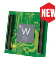
TEMPOROC Temporoc is a 64-channel front-end ASIC designed to readout silicon photomultipliers (SiPM) in particle time-of-flight (TOF) measurement applications.
