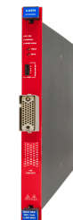
Single width (5 TE wide) - REDEL 51-pin, 24/36/48 channel: A7030LPR, A7030LNR, A7030TPR, A7030TNR, A7030YNR, A7030YPR, A7030NR, A7030PR
