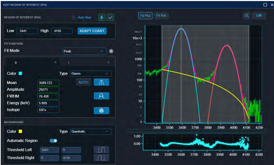
SmartMCA - The Edit Region of Interest window with the double Gaussian performed fit
