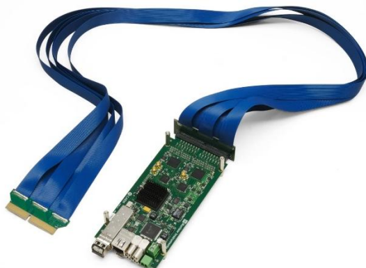
Fig. 3.3: FERS remotization cable
