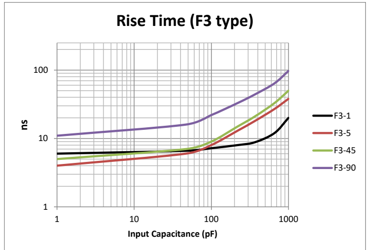
Fig. 2: Typical rise time vs. input capacitance (test input rise time = 1.6 ns; amplitude: 200 mV into 50 Ω).
