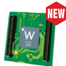
PSIROC Psiroc is a 64-channel front-end ASIC designed to readout PIN diodes, silicon strips and GEMs, handling detector capacitances ranging from 0 up to few hundreds of pF.
