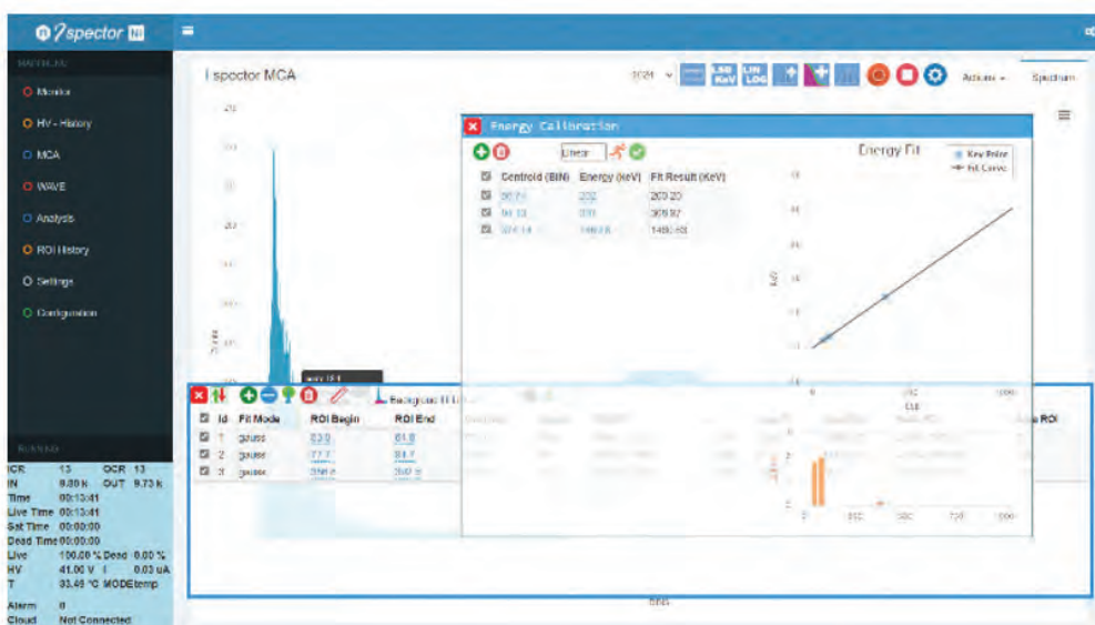
Linear dependency in the Energy Calibration.
